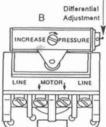
Note: Reverse action switches close (cut-in) on rising pressure.
